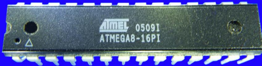
Microcontrollers are Integrated Circuits (ICs). They can have 6, 8, 14, 20, 28, 40, 64 or 100 pins.
