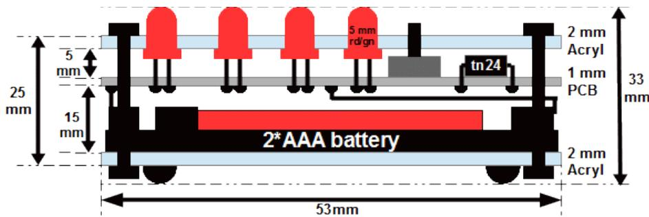
This is the side-view on the mounted device. It shows the acrylic glass casing on top and on the bottom and how the controller, the LEDs, the buttons and the AAA batteries fit into that. The bat-
